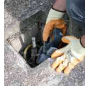
Elliptical jaw improves access
